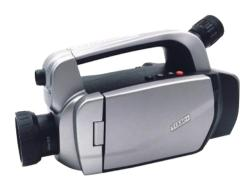
**TI330+** is with cooled detector (T2SL, NETD<25mK) to detect CH4 gas leaks and and pinpoint the gas leaks location accurately, also offers temperature measurement. It is a multifunctional device for gas leakage detection and thermograph applications.
