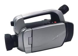
**TI320+** is with cooled detector(QWIP, NETD<25mK) to detect SF6 and NH3 gas leaks and pinpoint the gas leaks location accurately, also offers temperature measurement. It is a multifunctional device for gas leakage detection and thermograph applications.
